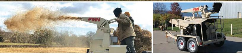
FINN Straw Blowers multiply your productivity and profits by doubling straw coverage in a fraction of the time it takes to apply by hand. There's no more efficient way to ensure soil moisture retention and protect against erosion damage to freshly seeded areas.
