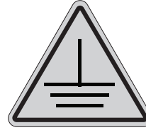
Grounding Required Hazard
