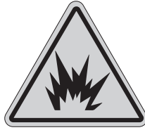
Arc Flash Hazard or Explosion Hazard
