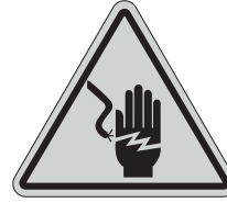
High Voltage Hazard
