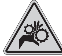
Pinch Point/ Entanglement Hazard
