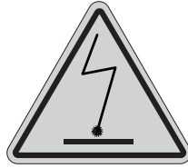
Electrostatic Discharge Hazard
