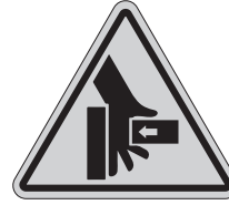
Crush/ Entrapment Hazard
