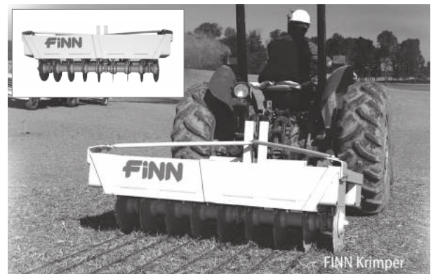
6 ft. 3-point hitch Krimper shown. 8 ft. 3-point hitch is similar with 12 blades.
