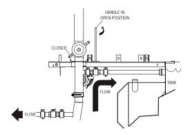
Figure 7 – Discharge Through Extension Hose or Hose Reel
