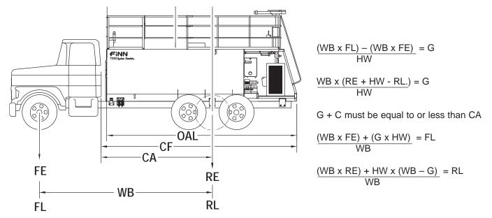
Figure 1 – Truck Mounting Calculations and Dimensions
