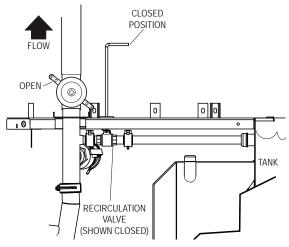
Figure 6 - Discharge Through Boom
