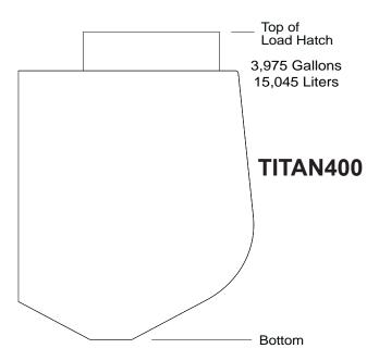
Figure 16 – Tank Capacity Chart (Sheet 2 of 2)
