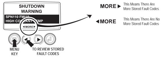
Figure 15 - Stored Fault Codes
