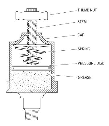
Figure 1 – Automatic Pressure Lubricator Components
