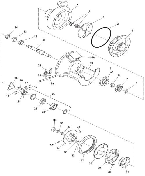
Figure 8 - Clump Assembly Components
