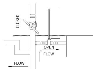
Figure 5 – Discharge Through Extension Hose or Hose Reel Through Remote Port
