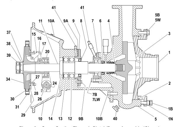
Figure 9 – Cross-Section Through Clutch/Pump Assembly (Clump)
