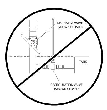
Figure 2 - NEVER Engage Slurry Pump Clutch w/ Both Valves Closed
