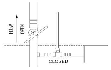
Figure 4 – Discharge Through Boom or Extension Hose Through Boom
