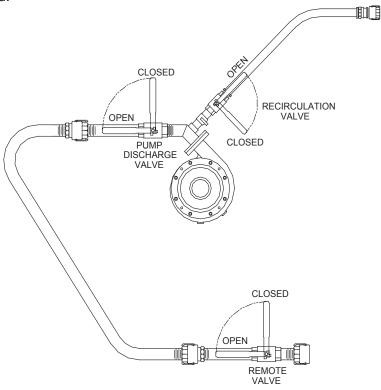
Figure 2 - Valve Operation
