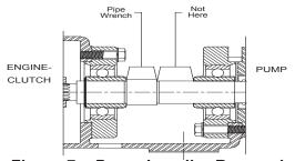
Figure 7 - Pump Impeller Removal
