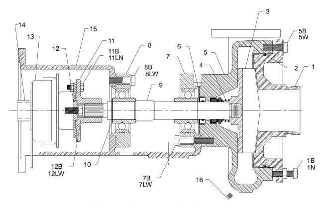
Figure 6 – Pump Assembly Components
