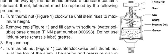
Figure 1 **Automatic Pressure** Lubricator
