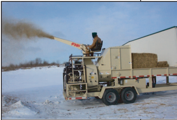
Straw Blower Winterizing
